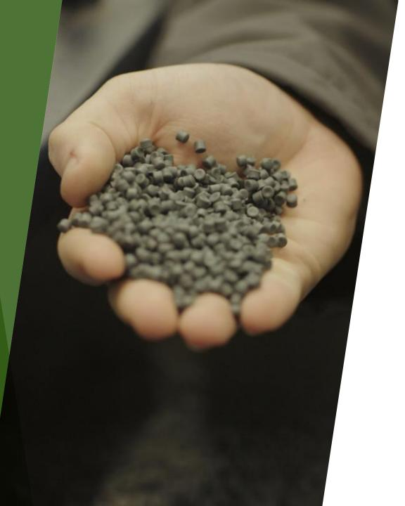
Once shredded and cleaned the Aky print is then extruded and any waste in removed before being pelletized:
