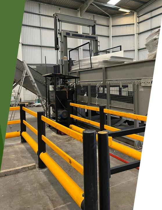
These bales of Aky Print are loaded directly onto a conveyor where they pass under a guillotine and are chopped down to approx. 1 foot in length:
